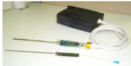
FIGURE 2. Probe, consisting of matching box, cable, probe handle (cover removed) and transducer module. A second module is shown removed from the quick-disconnect handle.
