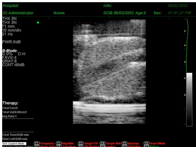
Figure 7. Imaging results from a prostate phantom using 3.4 MHz, 3.4 \lambda_0 pitch, 32 element probe. Image depth is 71 mm and width is 50 mm. Quantitative studies show resolution and contrast are comparable to transabdominal probes at a depth of 50 mm [2].
