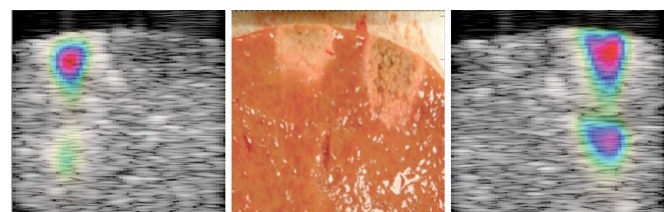
Fig. 4. Echo difference maps and thermal lesions obtained using a 64 element, 6 MHz image-treat array for two thermal ablation experiments. Each panel shows a region of width 38 mm and height 37 mm. The left and right echo difference images, superimposed on B-scans obtained using the same probes, correspond to the left and right lesions shown in the center panel. The echo difference is displayed by linearly scaling image hue and saturation such that red corresponds to the maximum value and transparency corresponds to the minimum value.
