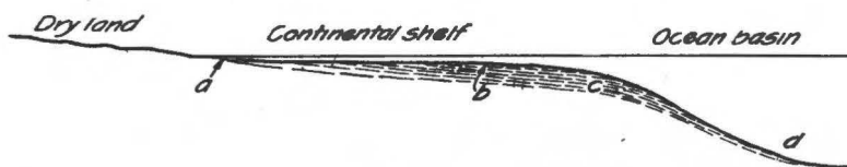
Fig. 15.—Diagram showing continental shelf and edge of ocean basin. These slopes are at least five to twenty-five times as steep as in nature. a —coarser sediments; b —finer sediments and organic deposits; c —edge of continental shelf approximately 600 feet deep; d —thin deposits of very fine mud and organic remains.
