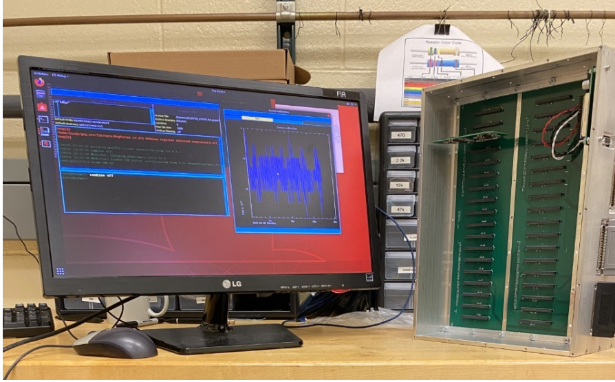
Figure 7: A picture of the general set-up. The computer screen on the left of the photo shows the GCP. The silver box with the motherboard is the Backpack. Inside the backpack you can see the motherboard with a daughter card inserted into a slot. Each of the black spaces on the motherboard are the "slots" referred to above.
